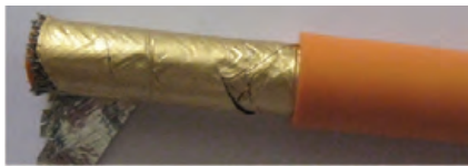
Fig. 67. Layered shield: braided shield with aluminium foil wrapped around it
