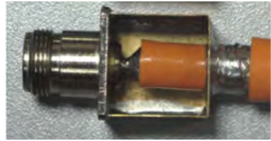
Fig. 70. Cable termination with adapter and N-type connector
